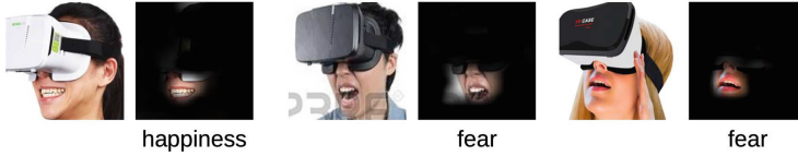
Fig. 1. Images (of people wearing VR headsets) with corresponding Grad-CAM [28] explanation masks and labels from a VGG-face model trained on lower-half images.
