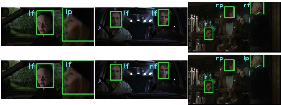
Fig. 5. Visualization of head orientation classification results using three examples. The top row shows the result of HoG + CNN features , and the bottom row lists the result of concatenated + spatial , which is able to correct misclassified results by local representation ( i.e. HoG + CNN features ).
