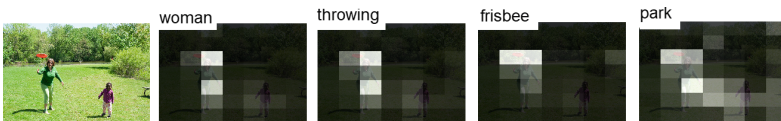
Fig. 4. Visualization of the attention over image regions while generating words “woman”, “throwing”, “frisbee” and “park”. The predicted sentence is “A woman throwing a frisbee in a park.”
