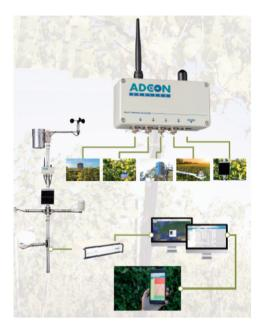
Fig. 1. Architecture of the ADCON telemetry
