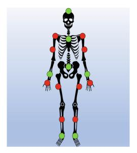
**Fig. 2.** [21] IMUs placed on the body (green dots: planned to be used in BauPrevent; red dots: usually used but planned to be neglected in this project). (Color figure online)
