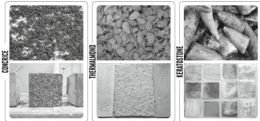
Fig. 10.1 Specimens manufactured from agricultural by-products and waste. From left to right: CONCRICE; THERMALMOND; KERATOSTONE
