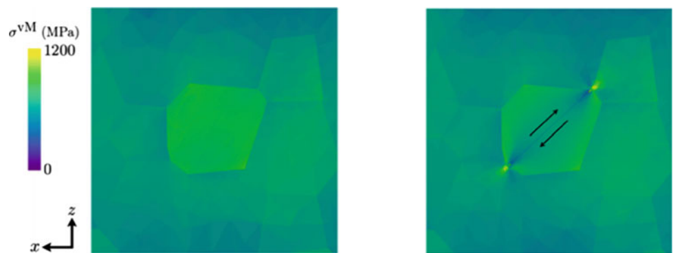
Fig. 2 Von Mises stress field prior to and post-twin activation (reproduced from [6])
