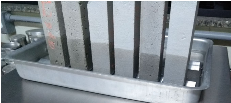
Fig. 3 Capillary rise of specimens 60 min after contact with water. Source Own author
