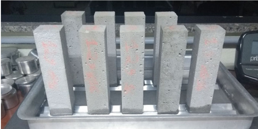
Fig. 2 Capillary rise after the specimens come into contact with water. Source Own author
