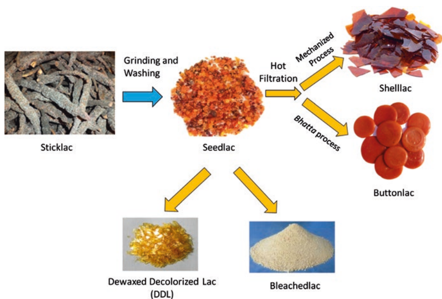
Fig. 1 Schematic diagram of processing of lac and its related products
