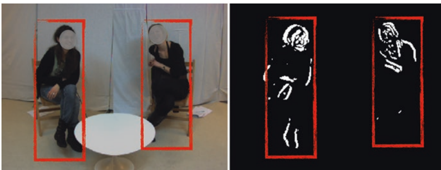
Fig. 1 The principle of Motion Energy Analysis (MEA). All pixel changes within the original video recording (left panel) of an interaction scene are highlighted (right panel). The rectangles delimit the respective regions of interest
