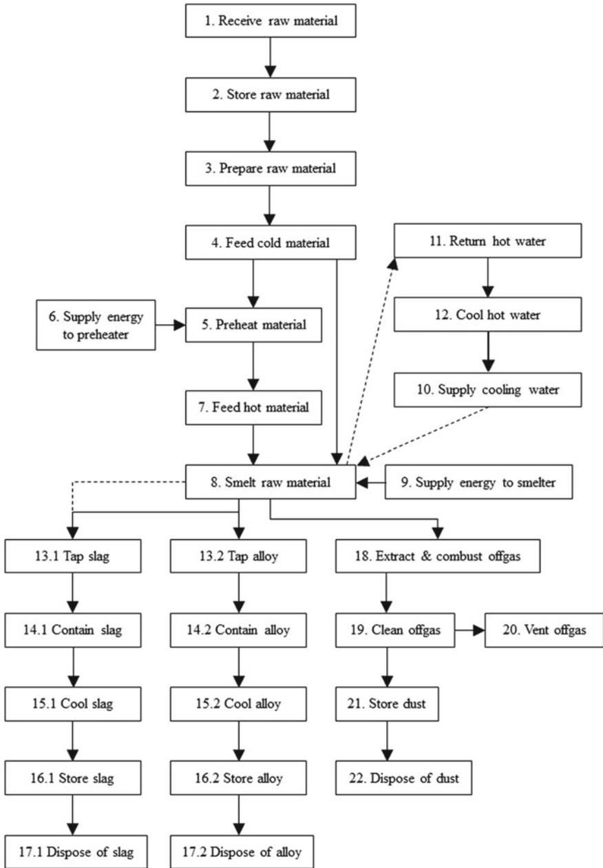
Fig. 1 Block flow diagram of the new facility
