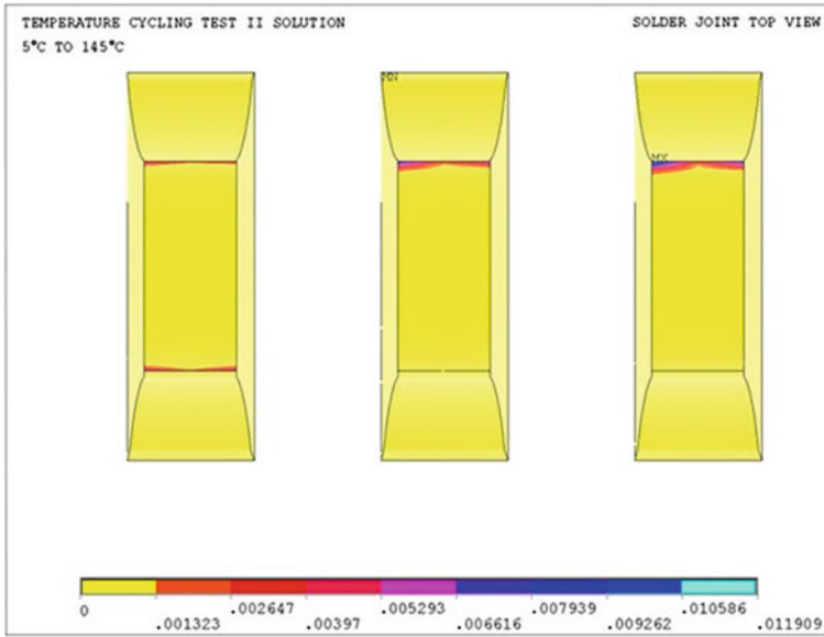
Fig. 9 Plastic strain in solder joints for ALT II (Top view)
