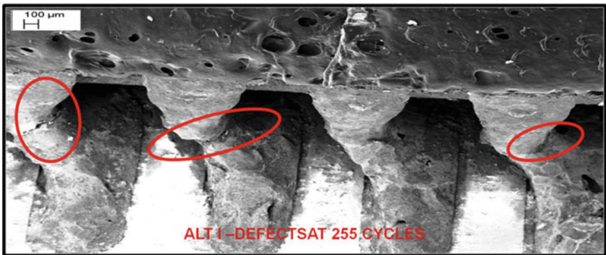
Fig. 23 SEM image of crack after 255 cycles for ALT I
