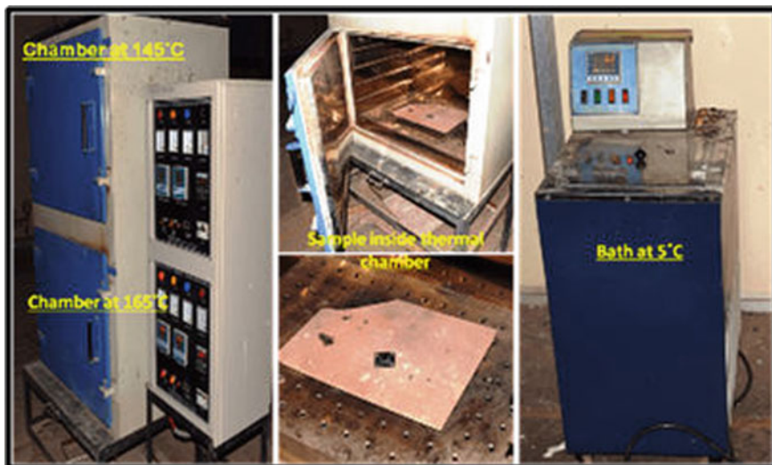
Fig. 16 Temperature cycling test set-up
