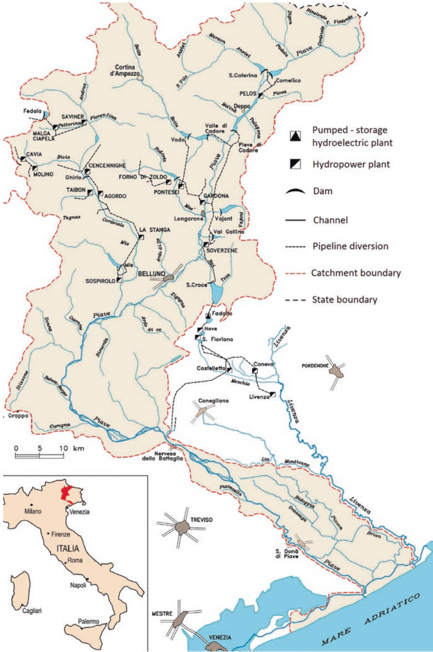
Fig. 2.7 Map of the Piave hydropower system
