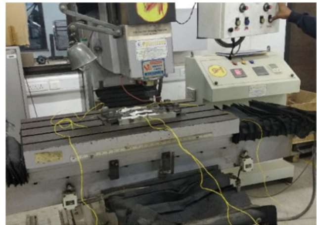
Fig. 2 Experimental set-up of FSW machine
