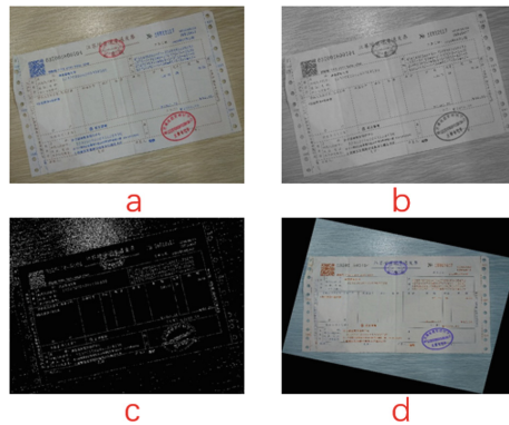
Fig. 7. Pre-processing process for invoice images in the experiment. a is the original invoice image; b is to convert the original image into a grayscale image; c is to convert gray image banalizations into edge image; d is the image obtained by the Hough transform and rotated.
