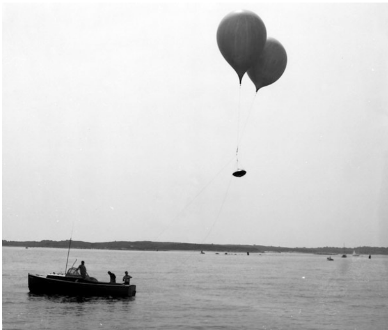
Fig. 14.10 Test of balloon-borne camera system over Vineyard Sound, MA. Note camera “capsule”, or gondola, suspended from two helium-filled fixed altitude balloons. If one balloon failed, then the camera bearing gondola would make a soft landing on the sea surface. (From author’s photo archive, circa 1969)
