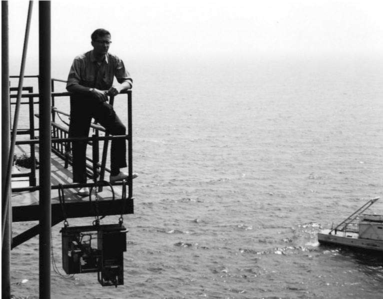
Fig. 14.8 The NMU Whitecap Camera System suspended beneath the deck of the Buzzards Bay Entrance Light Station. (From author's photo archive, circa 1968)
