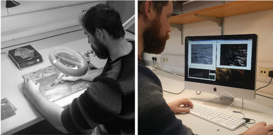
Fig. 2.2 Illustrations of the efforts involved in processing filmographic images using “cutting and weighing” method (Monahan 1969) (left), and for processing digital images using greyscale thresholding techniques (Monahan and Lu 1990)
