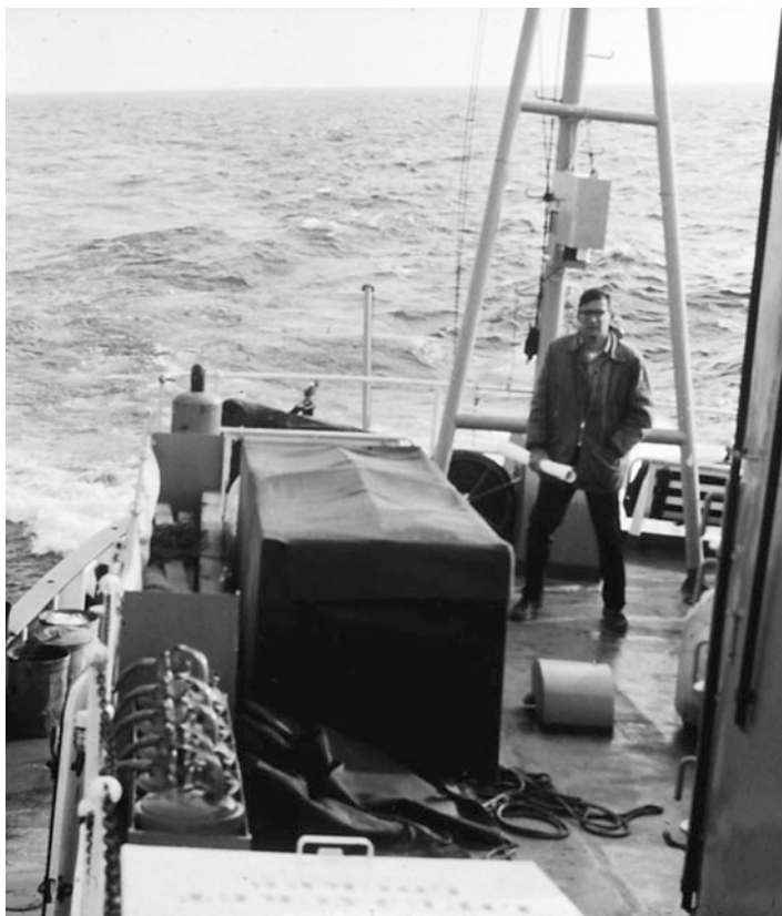
Fig. 14.7 Whitecap Camera System suspended so that it could move about a fore and aft axis in the rigging of the USCGC Naugatuck. (From uncopyrighted report, Monahan and Zietlow 1968)
