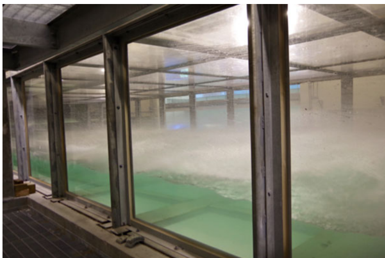
Fig. 10.5 SUSTAIN facility in operation at hurricane wind speeds, here with fresh water. Video impression from the wind ramp up to the highest wind speeds in the Kyoto and SUSTAIN facilities are in these videos: https://www.youtube.com/watch?v=KDcAzL01LT0 and https://www.youtube.com/watch?v=DUrP-rRnRxU
