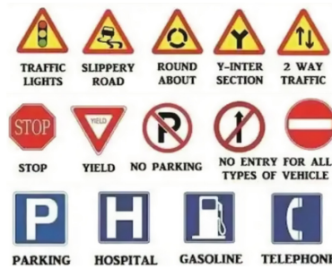
Fig. 1. Example of traffic signs classes: (from top to down) danger proclamation signs, regulation signs, and informational signs (Color figure online)
