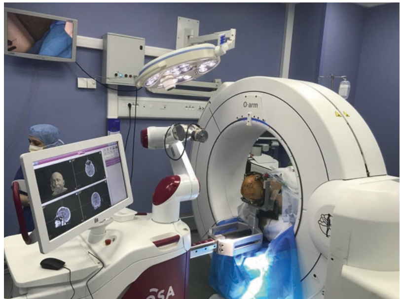
Fig. 4.5 Robot-guided surgery performed at Grenoble University. The head of the patient is rigidly fixed using a head holder (here, a Leksell Frame). The patient is installed into an intraoperative scan (Oarm, Medtronic) that allows intraoperative image verifications of lead placements
