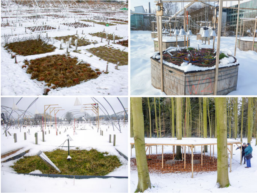
Fig. 4 Examples for winter climate change manipulation experiments. Top left, soil warming by heating wires in the ground to avoid soil frost come with the drawback that soil warming in the absence of air warming is unrealistic (Schuerings et al. 2013); top right, ecosystem warming by infrared heaters and warming cables on the ground allow for simulation of winter warming extremes as they are able to melt even thick snowpacks quickly (Kreyling et al. 2015b); bottom left, aboveground infrared warming mimics a warmer climate with realistic consequences on snow cover and soil temperature variation (Walter et al. 2013); bottom right, snow-out shelters reduce winter soil insulation while not altering water and nutrient input as the snow accumulated on the top melts through the perforated plastic sheets upon melting events (displayed study unpublished but see Kreyling et al. 2012a for comparable setup). Combining snow-out shelters with realistic changes in winter precipitation amount and/or air temperature warming is a promising approach to test for winter climate change effects in temperate ecosystems
