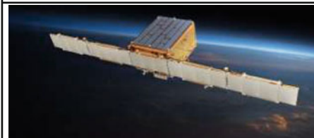
Figure 3g: Planar patch array that flew on Iceye X1 satellite. Graphics courtesy of Iceye.
