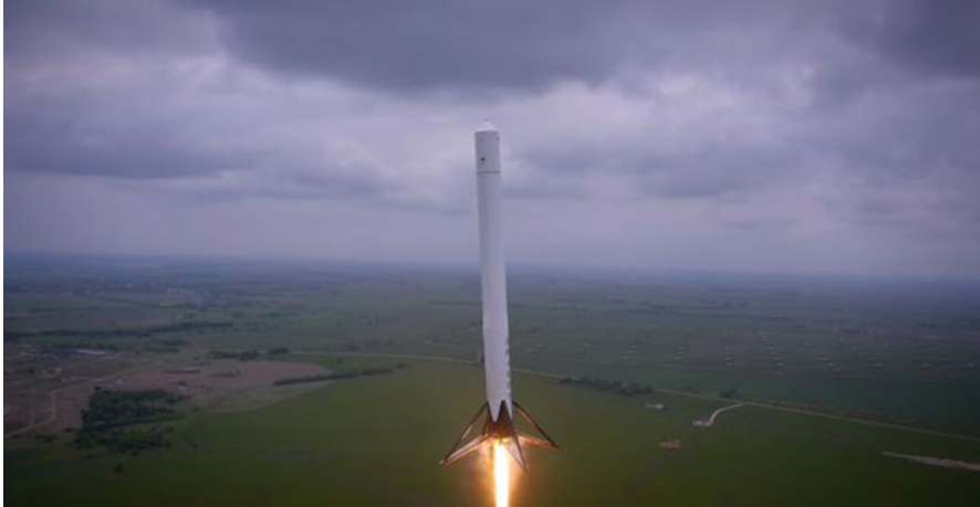
Fig. 4 Test flight of the Falcon 9 Reusable (F9R) launcher that promises new economies for smallsat launches. (Graphic courtesy of SpaceX)
