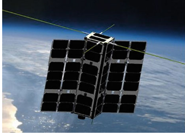
Fig. 3 Lemur 2 nanosat with payloads for AIS, ADS-B, and weather data. (Graphic courtesy of SPIRE Global Inc.)
