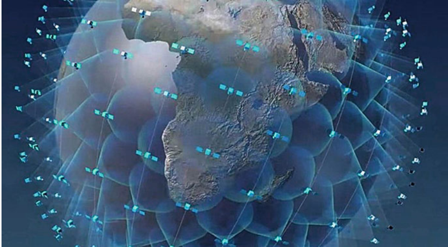
Fig. 4 OneWeb representation of its LEO constellation, upwards of 600 satellites at 1200 km in 24 individual orbital planes. One Web Small Satellite constellation (Graphic courtesy of One Web)
