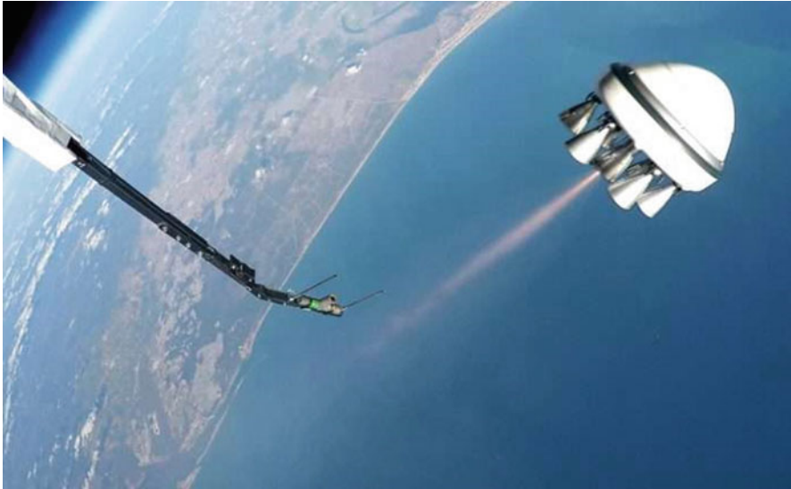
Fig. 7 Zero 2 Infinity Bloostar rocket prototype deployed from a stratospheric balloon. (Credit: Zero 2 Infinity)
