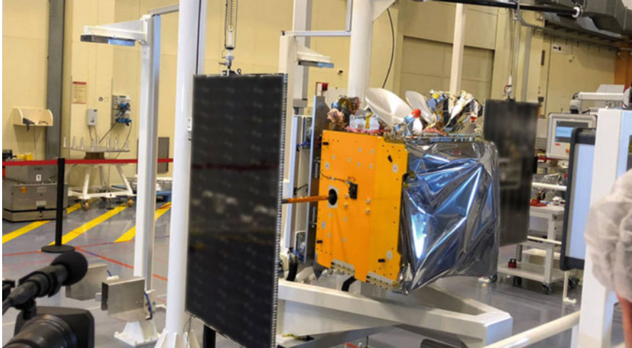
Fig. 3 One of the 110 kg. OneWeb satellites in production in Toulouse, France. (Graphic courtesy of Airbus)
