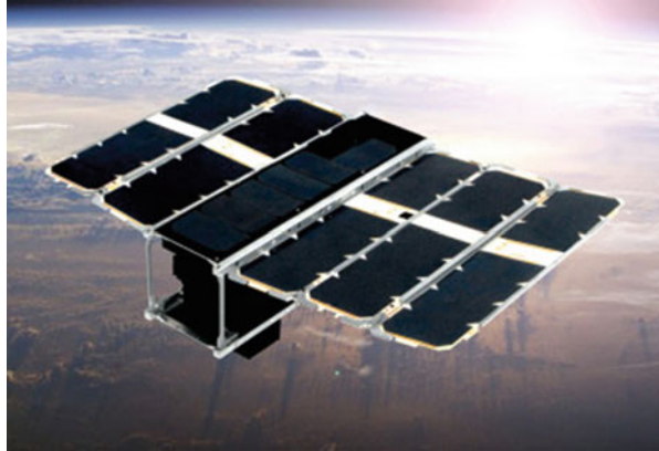
Fig. 4 The 3-unit cube satellite SENSE experimental project for US Air Force. (Graphic courtesy of the US Air Force)
