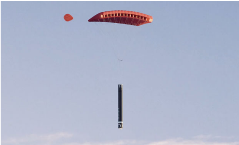
Fig. 17 A rendering of Electron's first stage with chute deployed for reentry, awaiting air capture by helicopter. (Graphic courtesy of Rocket Lab)
