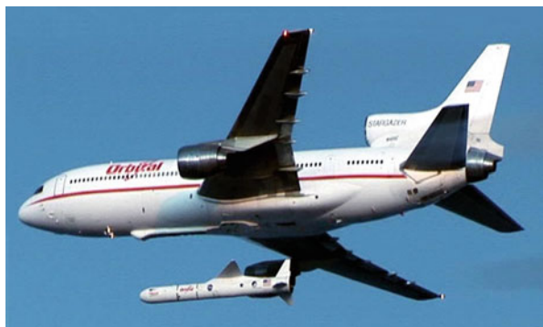
Fig. 4 The Orbital Sciences L-1011 jet aircraft releases the Pegasus rocket carrying the Space Technology 5 spacecraft with its trio of microsattellites (2006). (Graphics courtesy of Northrop Grumman Innovation)
