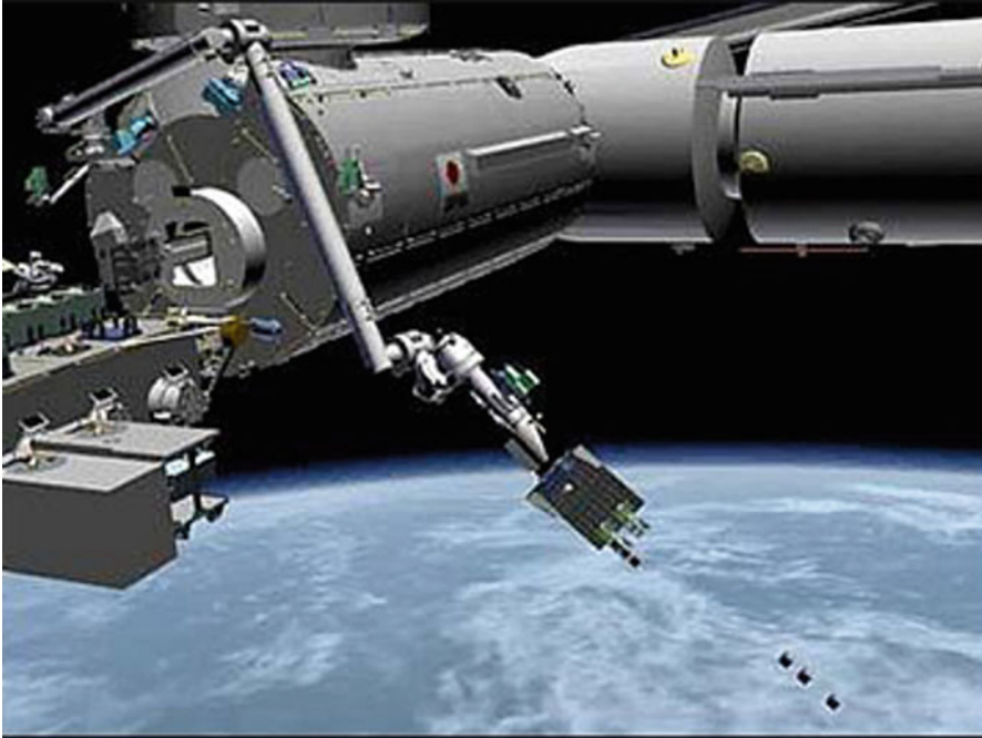
Fig. 4 The J-SSOD on the ISS deploying three 1U cubesats. (Images courtesy JAXA)
