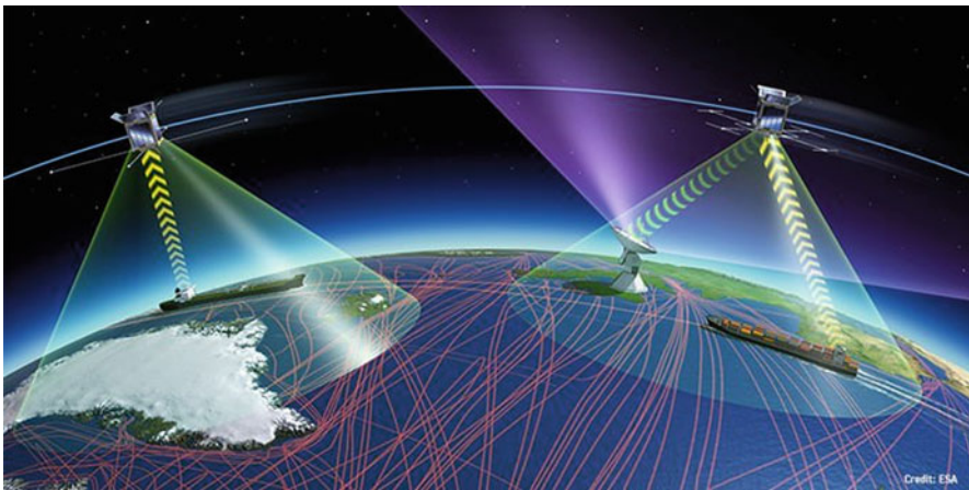
Fig. 2 Graphic showing satellite reception of S-AIS signals from ships on the high seas. (Graphic courtesy of the European Space Agency)
