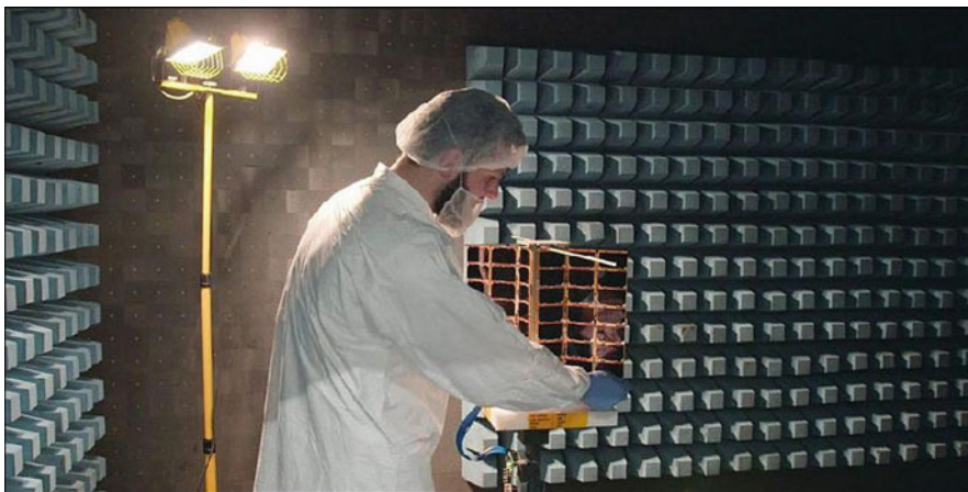
Fig. 11 A Spire technician manipulates a LEMUR2 satellite in Spire's EMC chamber. (Graphic courtesy of Spire, ©Spire Global)
