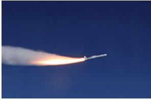
Pegasus in flight after release from Lockheed 1011 Carrier Aircraft (Graphic courtesy NG Innovation)
