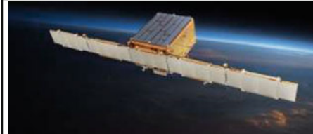
Figure 3g: Planar patch array that flew on Iceye X1 satellite. Graphics courtesy of Iceye.
