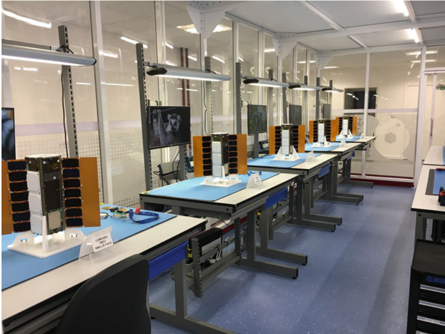
Fig. 9 LEMUR2 satellites in the Spire cleanroom. (Graphic courtesy of Spire, ©Spire Global)
