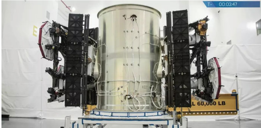
Fig. 4 The TinTin prototype satellite for technology verification for the Starlink constellation. (Graphic Courtesy of SpaceX)
