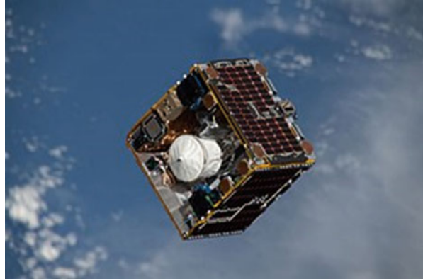
Fig. 5 The RemoveDEBRIS small satellite in orbit. (Graphic Courtesy of Surrey Space Centre)
