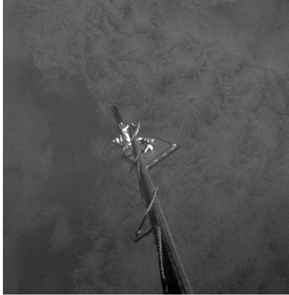
Fig. 24 Target retained by harpoon tether wrapped around the boom
