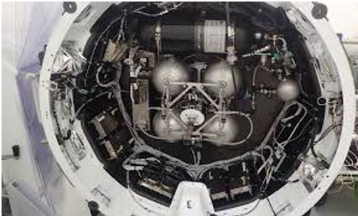
Fig. 5 Electron's Kick Stage during final prelaunch fit-out. (Graphic courtesy of Rocket Lab)
