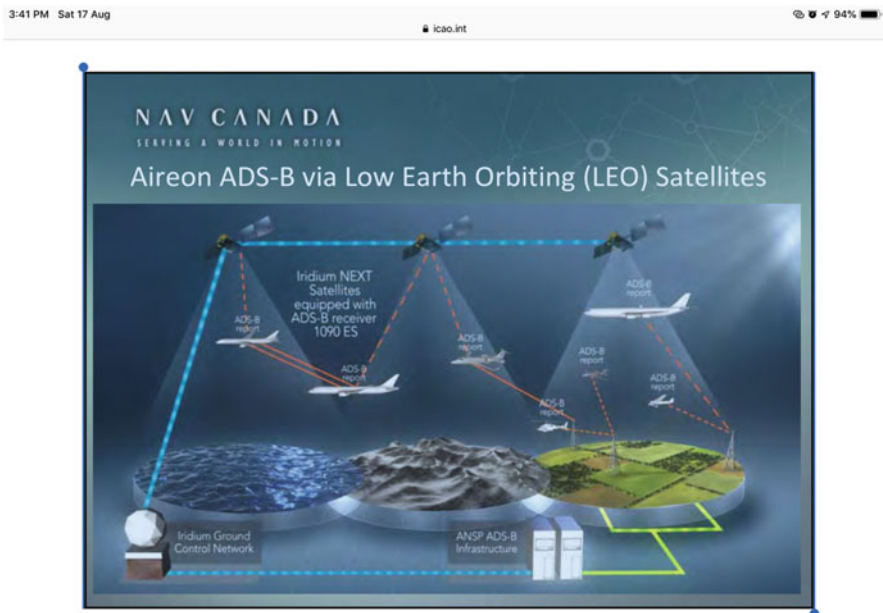
Fig. 1 Operational configuration between aircraft and Aireon packages. (Graphic courtesy of NAV Canada)
