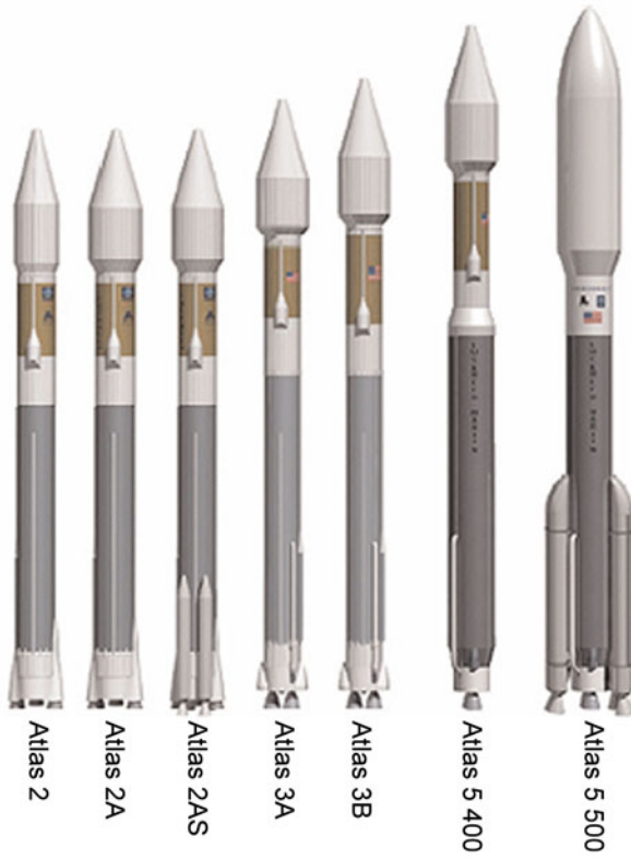
Figure showing the relative size of the Atlas II, Atlas III, and Atlas V 400 and 500 series. (Graphic Courtesy of the Wiki Global Commons)
