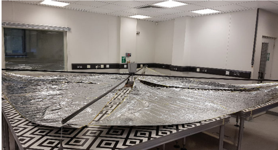
Fig. 28 Ground testing of the DragSail for the SSO-A mission
