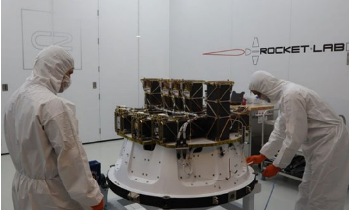
Fig. 7 13 CubeSats for the NASA ELaNa-19 mission in December 2018 being integrated onto the Kick Stage in preparation for launch. (Graphic courtesy of Rocket Lab)
