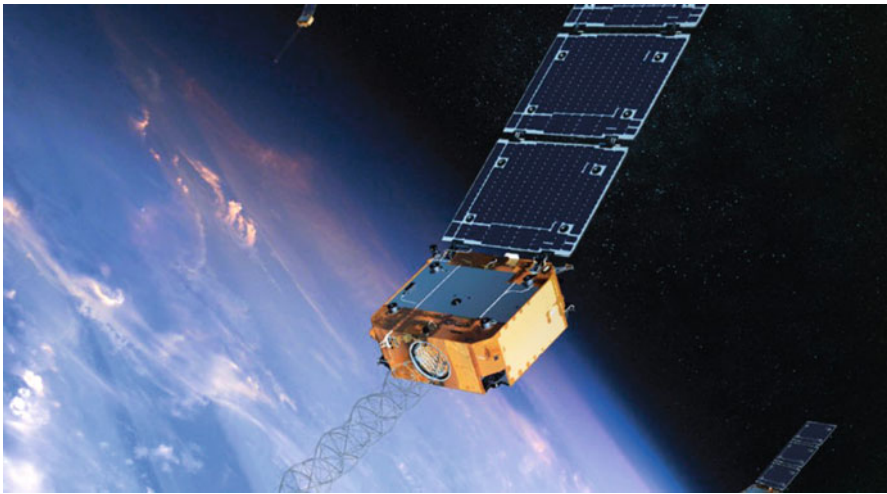
Fig. 5 The OG2 ORBCOMM satellite with an L-band package for messaging services. (Graphic courtesy of ORBCOMM)
