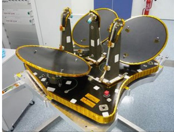
Fig. 2 The Q/V Aldo Paraboni experiment payload that rides aboard the Alphasat project by ESA (Graphic courtesy of ESA)
