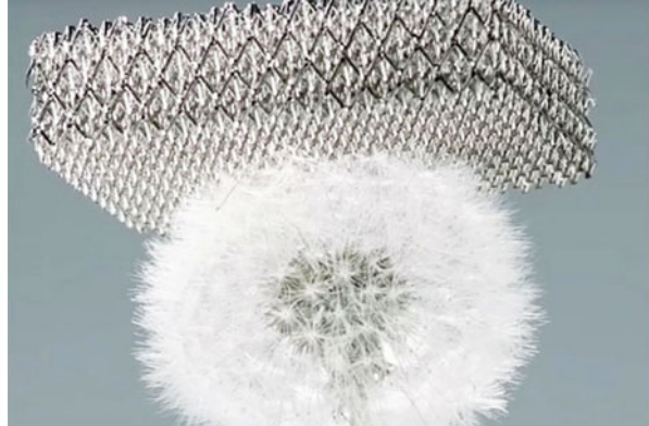
Fig. 3 A super low mass micro-lattice variant suspended on top of a dandelion. (Graphic courtesy of Boeing)
