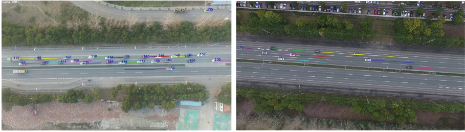
Fig. 8. Illustration of vehicle tracking in drone video. The line following the vehicle is the trajectory of the vehicle.
