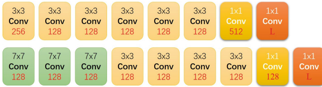
Fig. 3. Detailed kernel size and channels of convolution layers in Conv in Fig. 2, the first row is Conv(stage1), and the second row is the Conv(stage>1). The L in last layers denote the number off facial landmarks and mask.
