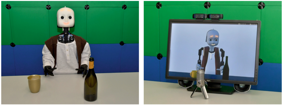
Fig. 1. Experimental setup of the two conditions: the physical robot on the left and virtual agent on the right. Participants sit at the table in front of the respective agent.
