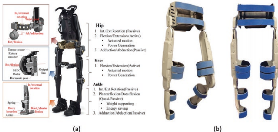
Fig. 8.11 (a) Structure of HEXAR-CR50 exoskeleton and joint modules [42]. (b) The structure of the Vanderbilt [26]
