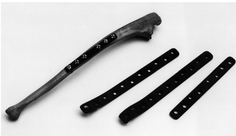
Fig. 2.5 Carbon fiber reinforced epoxy plates for epiphyseal fractures. (Courtesy: Elsevier and Orthodynamics, UK [31])
