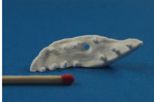
Fig. 9.21 Printed structure of a granulated bioglass- \beta -TCP granule [8]
