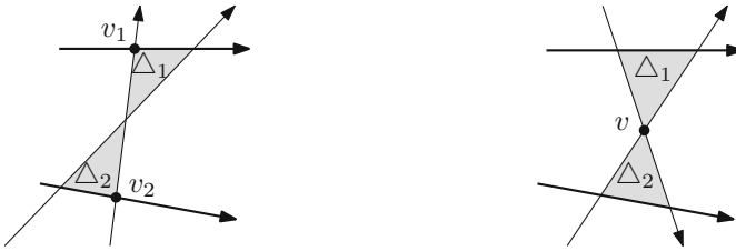
Fig. 6. Left: the two triangular cells \Delta_1 and \Delta_2 do not form an hourglass, because they share a vertex that is not an exit vertex. Right: the two triangular cells \Delta_1 and \Delta_2 form an hourglass because they share an exit vertex.
