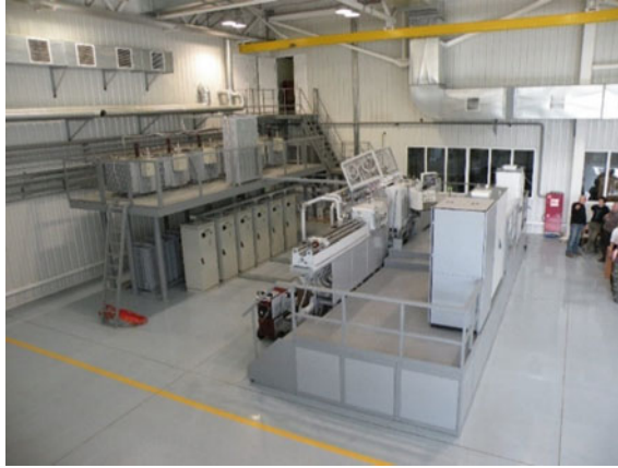
Fig. 4 TBC electron-beam unit L-8 (From The Paton Welding Journal, No. 5–6, 2016. Used with permission)
