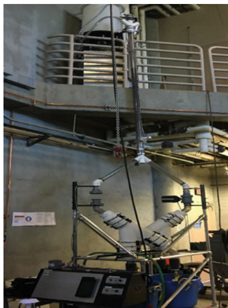
Fig. 2 Pilot-scale dual column continuous flow reactor (left). Flow diagram of the third generation dual column reactor (right) [7]
