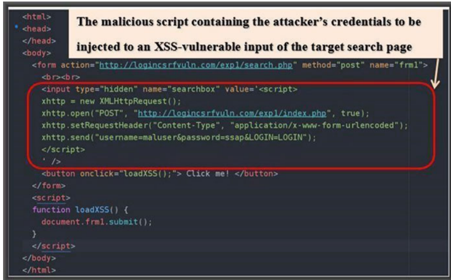
Fig. 3 The source code of the malicious page to exploit XSS in the search page
