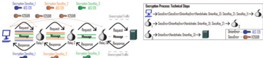
Fig. 9 Tor traffic encryption process
