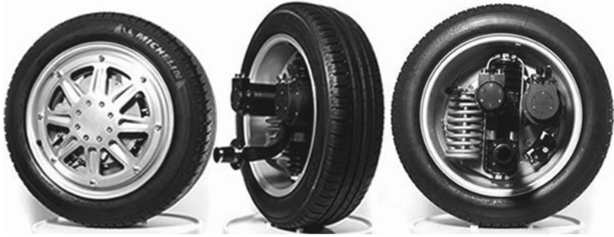
Fig. 28.4 The active wheel built by Michelin: a complete corner unit, provided with drive motor, brake, suspension and steering
