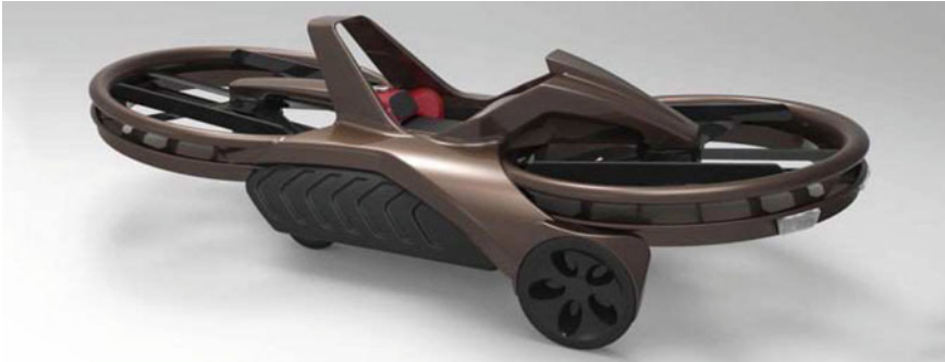
Fig. 28.12 The Aero-X hoverbike: a twinrotor vehicle, which is half way between a multirotor and a hovercraft
