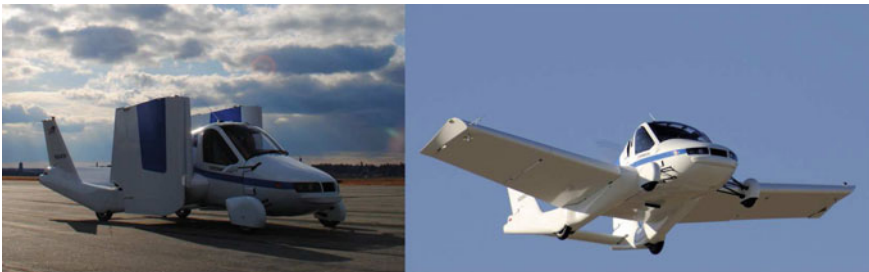
Fig. 28.7 The Transition ® , a roadable aircraft presented by Terrefugia at the 2012 New York Auto Show
