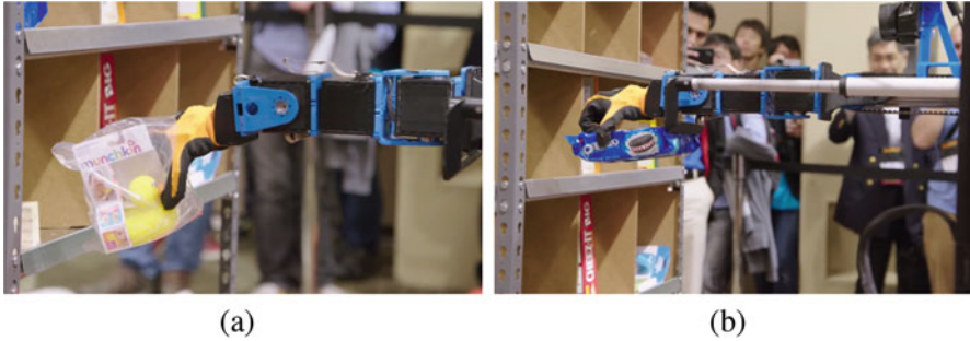
Fig. 9 (a) Example of picking up an object with Pisa/IIT SoftHand. (b) Example of picking up an object with the piston.
