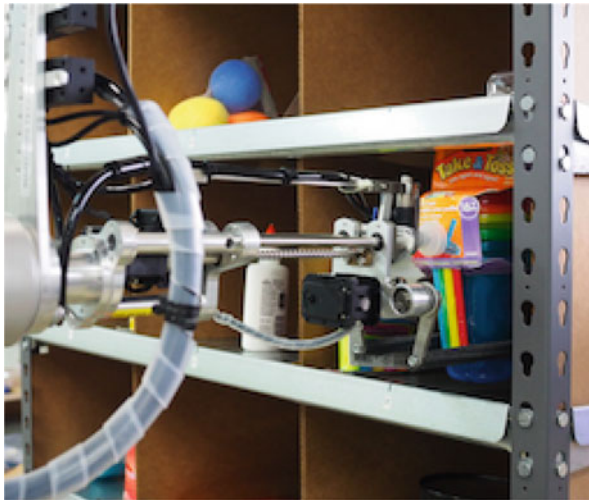
Fig. 3 A close-up of the Mantis gripper as it picks an item from the shelf. For this item, the gripper deployed both its suction and its parallel jaw gripper. The Kinect sensor is mounted at the end-effector, just above the gripper
