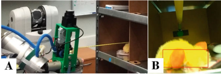
Fig. 7 Illustration of pulling routine. (a) the system extend the linear actuator to pull the yellow duck from region 3 to region 1. (b) Eye-in-hand view during pulling execution
