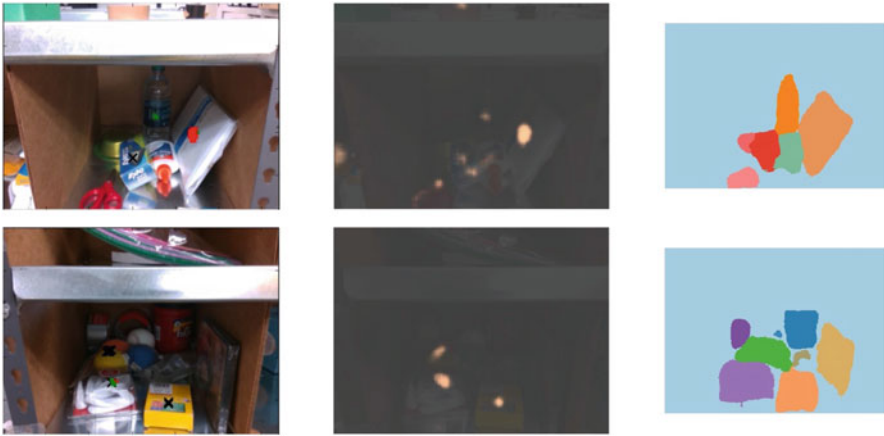
Fig. 5 Example of outputs produced by our network model containing (from left to right): (1) a color image with the selected grasp, (2) depth image with all available grasp candidates, and (3) semantic segmentation of objects in the scene
