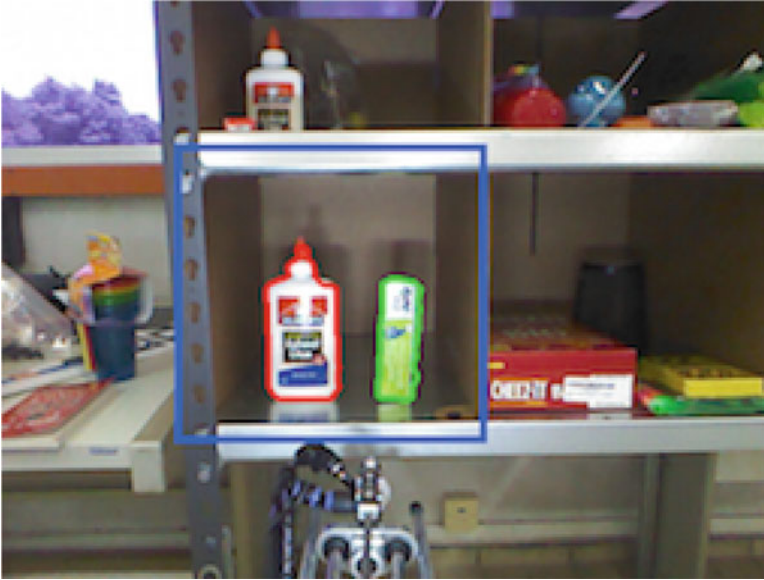
Fig. 4 Segmented objects from a typical image of the shelf bin. The blue rectangle denotes the region of interest (ROI) and the red and green contours display the segmented blobs, one of which could be the possible target object that initially have unknown identity
