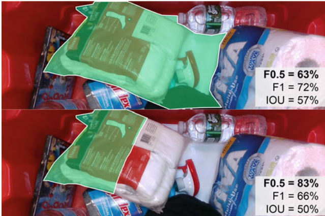
Fig. 8 An example illustrating the importance of different measures for grasping applications. Top: The object is undersegmented and the robot may pick a wrong item if a pick is executed in the segmented region. Bottom: only half of the entire object is segmented correctly. Yet F1 and IoU scores are very similar scores as in the above example. The F_{0.5} score is higher than in the above example. We argue the F_{0.5} is therefore more informative and more suitable for creating correct grasp points and successfully manipulate the objects. We argue that the F_{0.5} measure is more informative. Note that precision would also be indicative of success in this example, but should not be used in isolation because it loses information about recall
