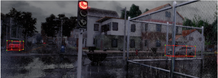
Fig. 3. Occluded vertices behind a chain fence. Note that both cars are visible, and thus have a bounding box drawn around them. Occluded and visible vertices are drawn with red and green, respectively (Color figure online).
