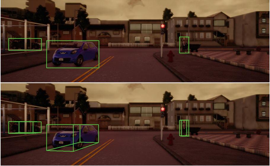
Fig. 2. 2D (top) and 3D (bottom) bounding boxes as generated by CADET. Class labels are omitted.
