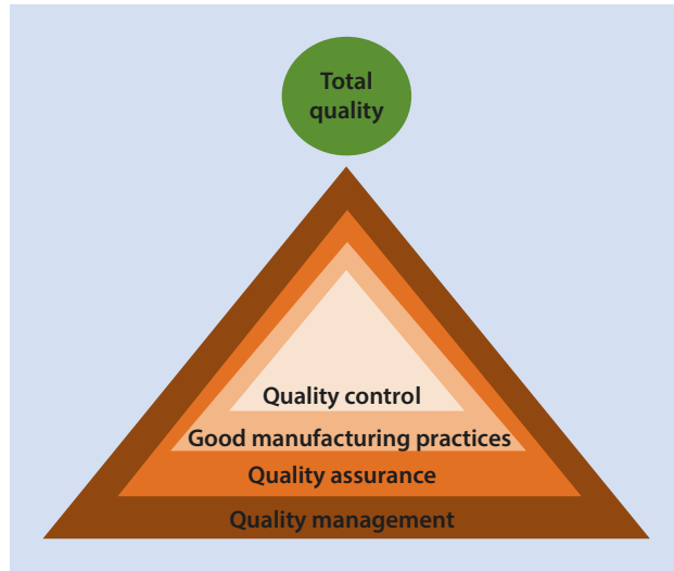
■ Fig. 6.1 Quality relationship. QM, QA, GMP, and QC are interrelated concepts. The main target of these concepts is to attain total quality
