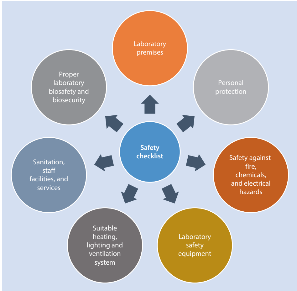
■ Fig. 3.2 Safety checklist. Important points which should be considered in the safety checklist of GLP [7]. To ensure proper establishment, there should be answer to questions about laboratory premises; staff facilities and services; safety against fire, chemicals, and electrical hazards and also suitable heating, lighting, and ventilation system; and more importantly laboratory biosafety and biosecurity
