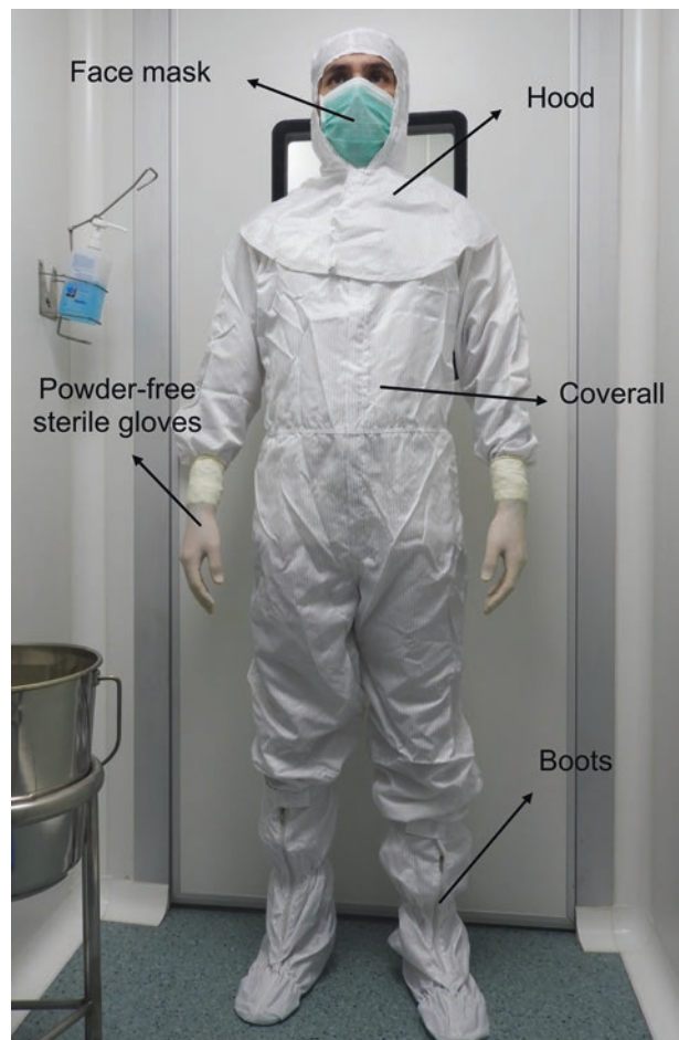
■ Fig. 7.2 Cleanroom suit. Personnel as one of the main sources of contamination must be trained and use the appropriate cleanroom suit. Appropriate cleanroom suit includes hood, safety glasses, face mask, main garment, sterile gloves, and boots
