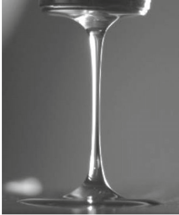
Fig. 35 Filament of the Newtonian silicon oil Wacker W1000 ( \sigma = 21.2 mN/m, \mu = 970 mPas) in a CaBER-type filament-stretching elongational rheometer (Stelter 2001)
