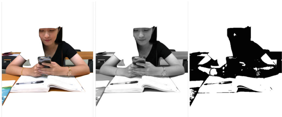
Fig. 2. Example result for pre-processing. The picture on the left is the result of removing the background, the image in the middle is the result after grayscale, and the picture on the right is the result of binarization.
