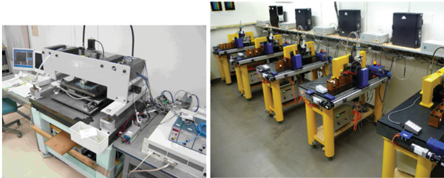
Fig. 9.10 Left: photograph of one of the Nagoya S-UTS scanning systems; right: the Bern scanning station equipped with five ESS microscopes with the associated automated film changers
