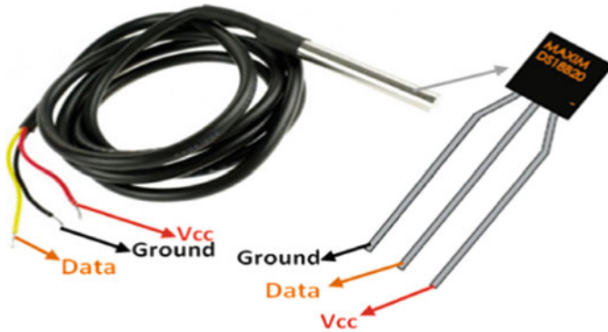
Fig. 7 Waterproof digital temperature sensor used for temperature sensing of soil. (Image downloaded from https://components101.com/sensors/ds18b20-temperature-sensor on May 29, 2019)
