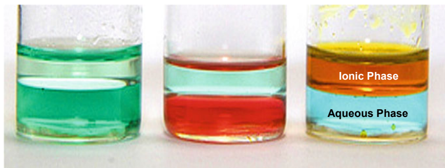
Fig. 7.10 A photograph of nickel(II) chloride (left), cobalt(II) chloride (center), and copper(II) chloride (right) dissolved in a water/[P 6 6 6 14 ][Cl]/ethyl ethanoate (4:1:1 v/v/v) biphasic solvent system. The upper phase is the ionic liquid [P 6 6 6 14 ][Cl]/ethyl ethanoate mixture and the lower phase is water saturated with ethyl ethanoate (7.6 wt%)
