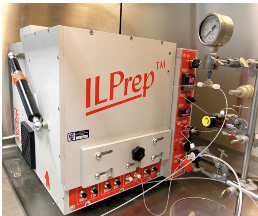
Fig. 7.3 The external view of a Quattro chassis CCC instrument (or IL-Prep™) instrument. For HPLC/HPCCC (high-performance liquid–liquid chromatography), solid supports are not used, and therefore the coil cannot clog up and result in inefficiency or damage because of impurities. If a new stationary phase is essential, more of the stationary phase is pumped in the instrument to regain the functionality of the coil
