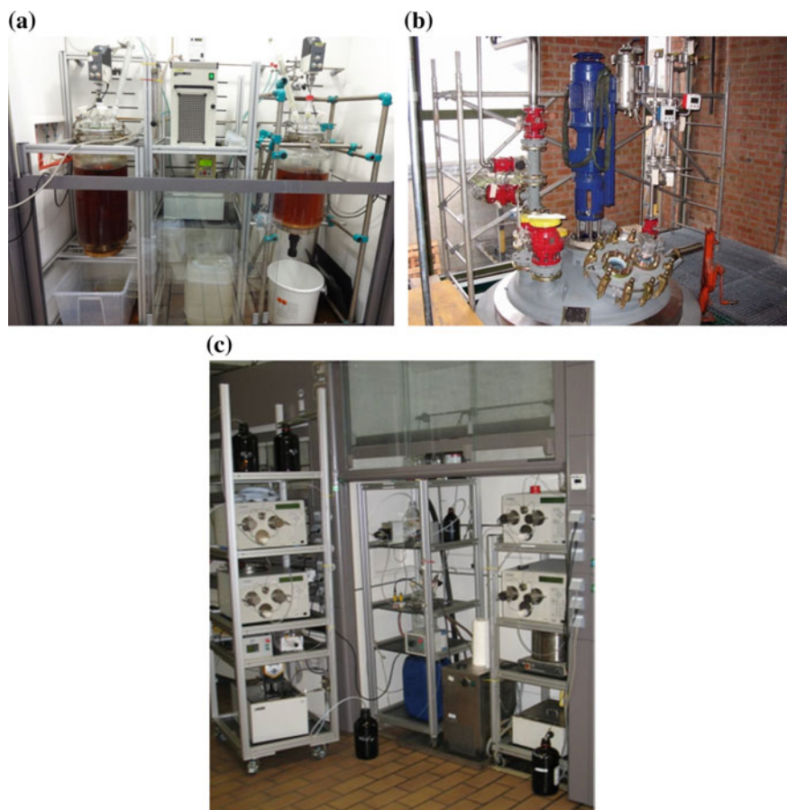
Fig. 8.1 (a) Glass reactors, batch size, 20 kg (© IOLITEC, 2019). (b) Stainless steel reactor, batch size 1 metric ton, operating pressure up to 10 bar (© IOLITEC, 2019). (c) Continuous-flow microreaction technology, 50 kg per day (© IOLITEC, 2019)
