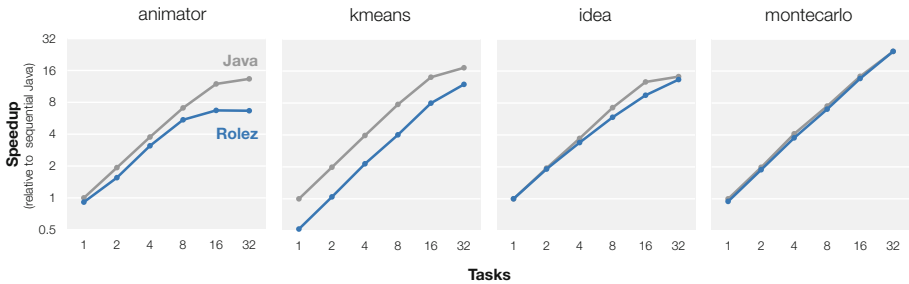
Fig. 10. Speedup of parallel Rolez programs, compared to speedup of parallel Java programs, for different numbers of tasks. All numbers are relative to single-threaded Java. Error bars are omitted since the variation is insignificant for all programs.
