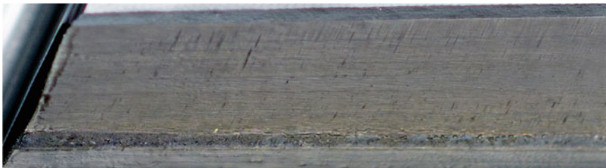
Fig. 9.30 Tooth surface damage photograph of the gear, No. = 14, N_P = 1.0 \times 10^6
