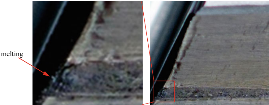
Damage to the tooth root at the end of gear engagement
