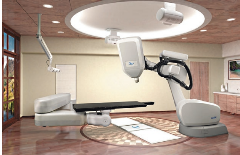
Fig. 4.1 CyberKnife system configuration showing the two X-ray cameras mounted on the ceiling. The two amorphous silicon detector imagers are embedded in the floor. (Image courtesy of Accuray Incorporated – © 2019 Accuray Incorporated. All Rights Reserved)
