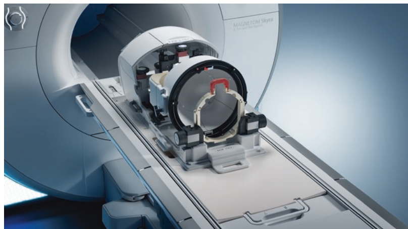
Fig. 16.4 ExAblate 4000 transcranial focused ultrasound system. (ExAblate 4000, InSightec). Patient is fixed to the table by a stereotaxic frame and a membrane holds water between the patient's head and the transducer. This transducer can be moved independently to target brain regions. (Image courtesy of INSIGHTEC)
