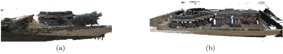
Fig. 8. 3D point cloud of (a) Bankapur Nageshwar Temple from original images (647 Images) (b) Bankapur Nageshwar Temple with our pipeline (139 Images).
