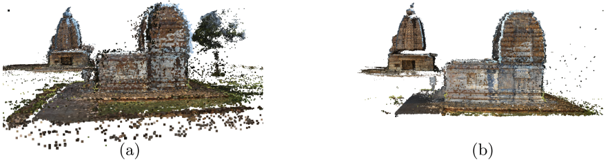
Fig. 9. 3D point cloud of (a) Pattadkal Temple from original images (220 Images) (b) Pattadkal Temple with our pipeline (92 Images).
