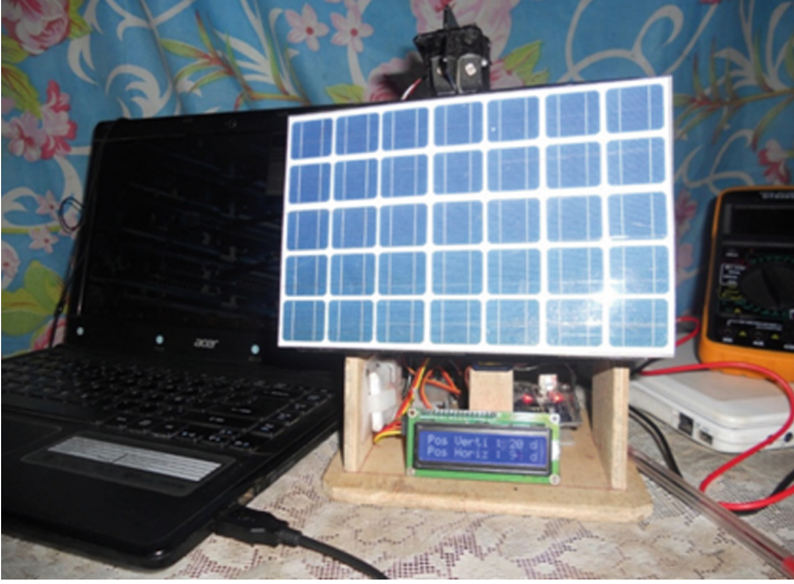
Fig. 5. Miniaturized implementation of the solar tracker
