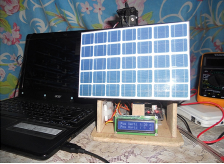
Fig. 5. Miniaturized implementation of the solar tracker
