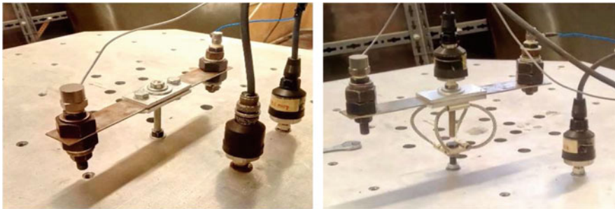
Fig. 5 Test setup for (left) the non-isolated structure and (right) the isolated structure
