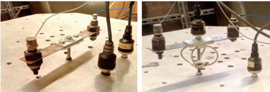
Fig. 5 Test setup for (left) the non-isolated structure and (right) the isolated structure
