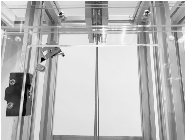
Figure 3. Elevator touch sensor.
