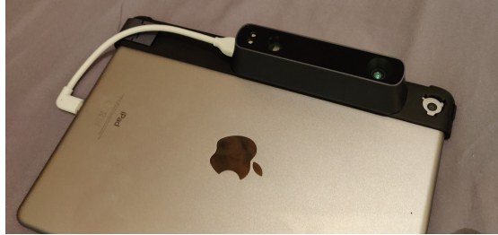
Fig. 1. The Structure Sensor mounted to an iPad
