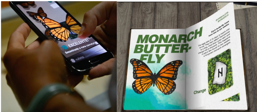
Fig. 4. Left side of the image: user interacting with the 3D model of the Butterfly displayed as Augmented Reality. Right side of the image: two pages of the digital book. It is possible to reload the 3D models of the animals by capturing the rune charms of the book pages.
