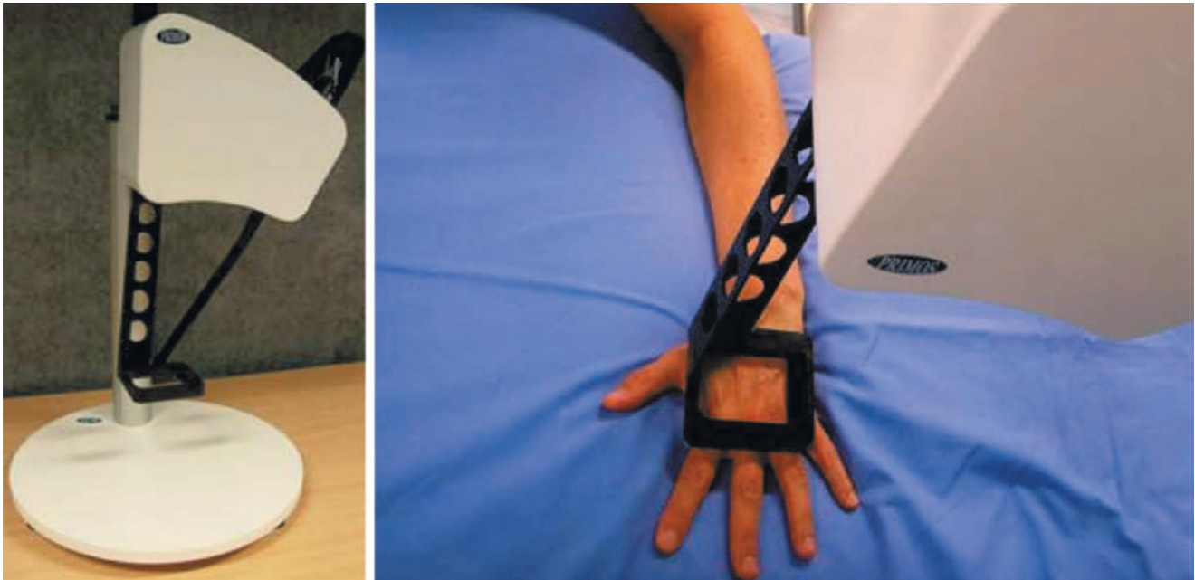
Fig. 17.5 Use of the PRIMOS in study patient. Upper left: The PRIMOS as objective measurement tool of scar surface roughness. Upper right: Use of the PRIMOS in the measurement of a scar on a hand. Middle left: PRIMOS live picture of scar treated with a substitute and a split-skin graft (substitute). Middle center: PRIMOS live picture of scar treated with split-skin graft alone (reference). Middle right:
