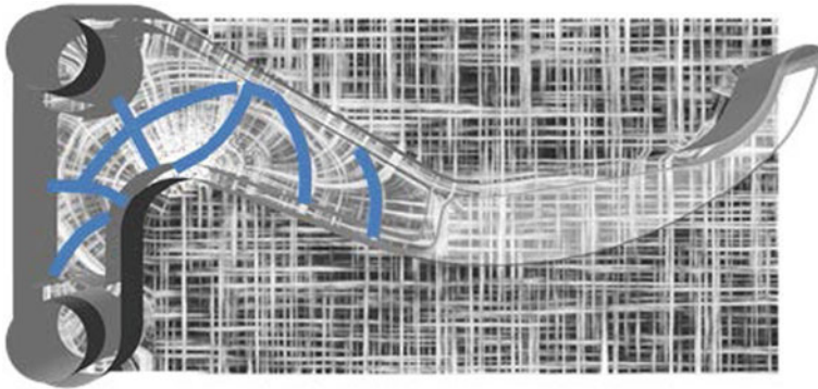
Fig. 13.4 Tensor fabric of the stress tensor in a planar cut through the CAD model. The engineer draws some lines manually to design rib support structures aligned with the tensor lines. These manual lines were the basis for the first new design. Two other drawings based on the same visualization led to the other two designs in our case study
