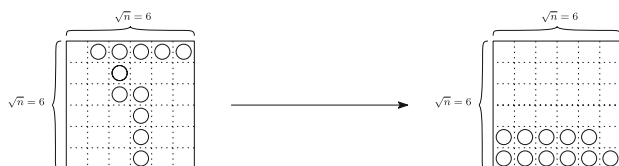
Fig. 3. An example of moving all nodes in a \sqrt{n} \times \sqrt{n} sub-box to fill in the bottommost rows of the sub-box (Phase A).
